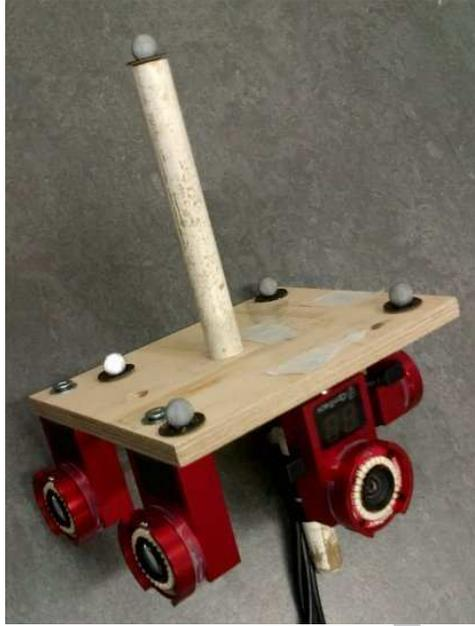
Figure 1: Multiple perspective cameras are arranged to form a camera cluster such that they cover as large an FOV as possible, even with no spatial overlap. This cluster consists of four cameras, two forward, one sideways and one backward-facing, at known positions and orientations.
