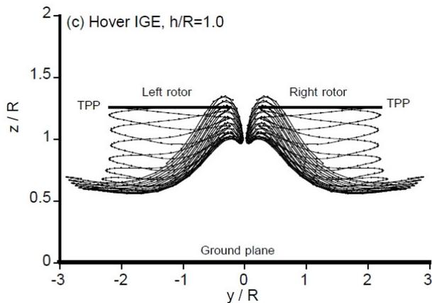
Fig. 9. Flowfield of Tandem Rotors in Ground Effect[4]
