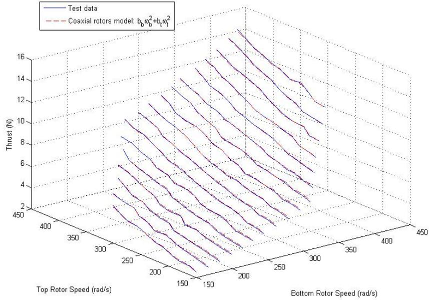
Fig. 5. Test data and fitted thrust model
