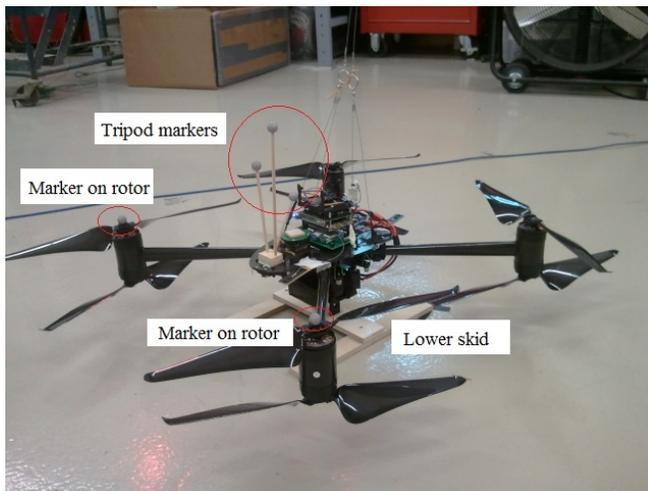
Fig. 3. X8 with lower skid and markers
