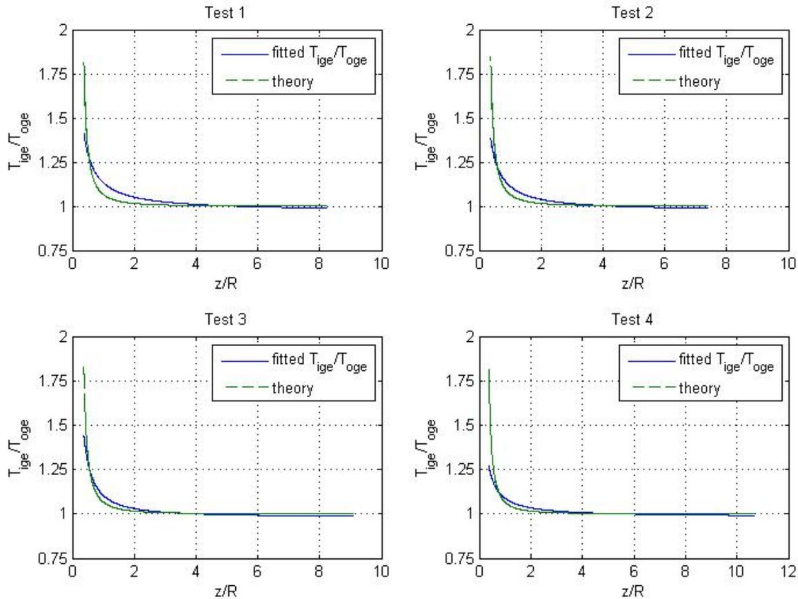
Fig. 8. Empirical GE vs. Calibrated Test GE
