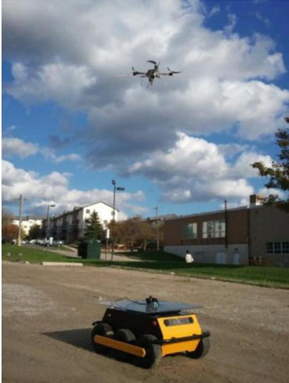
**Fig. 2.1** Quadrotor/UGV team performing coordinated landing [10]
