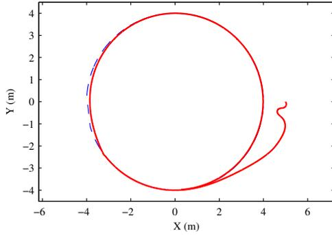
Fig. 1. Desired path (dashed) and trajectory of USV (solid) converging to and driving along desired path.
