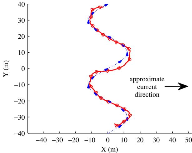
Fig. 4. Desired path (dotted) and trajectory of USV (solid) along commanded sinusoidal path measured in experiment using proposed controller.
