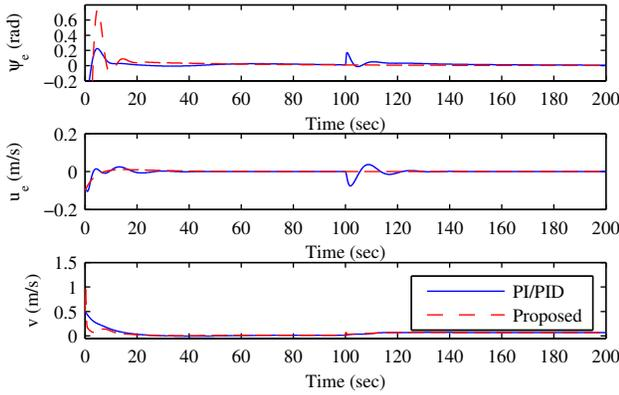
Fig. 2. Yaw tracking error  $\psi_e$ , surge velocity tracking error  $u_e$ , and sway velocity  $v$ . Dashed lines show results from controller presented here, while solid lines show results from a PI controller for surge velocity and a PID controller for yaw.
