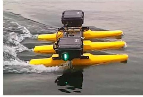
Fig. 3. The Clearpath Kingfisher M100 USV used in this work.
