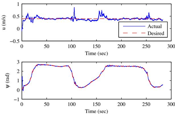
Fig. 5. Actual (solid) and desired (dashed) values for USV surge speed (top) and yaw angle (bottom) in experiment run using proposed controller.
