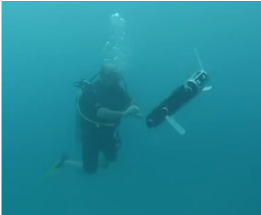
Fig. 8. Aqua robot during one of the open-sea autopilot trials at V = 0 , using the hovering gait. The robot was manually disturbed by the diver with a pitch angle of 45^\circ and then released.
