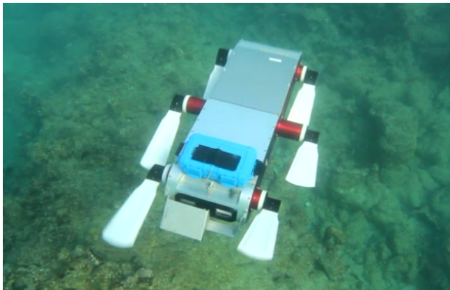
Fig. 1. Picture of the untethered Aqua robot used throughout the experiments in this paper. Photo credit: Y. Rekleitis.
