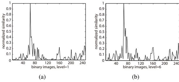
Fig. 5. This figure shows the similarity measuring based on MI between the 249th binary code and the previous binary codes at two different scales for the New College dataset. Level 1 represents the original image size (640x480), and level 6 is a down-sampled version by a factor of 32 in each image dimension (20x15).
