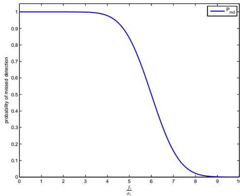
Fig. 2. Probability of a missed detection using the parity space test for a detection threshold of  $\delta = 6\sigma_e$ . Probabilities are computed as a function of the expected value of the fault vector magnitude, ranging from  $f_i = 0$  to  $f_i = 10\sigma_e$ .
