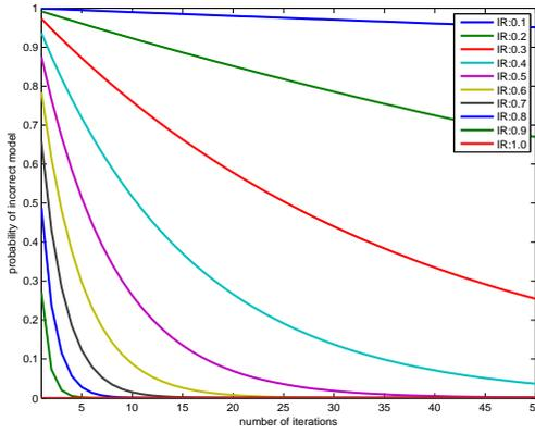
Fig. 1. Probability of RANSAC generating an incorrect model for  $c = 3$ . Probabilities are computed for inlier ratios ranging from 10% to 100% (IR:0.1 to IR:1.0).
