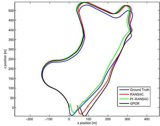
Fig. 6. Vehicle motion generated using visual odometry and outlier rejection techniques for S05.
