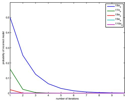
Fig. 3. Probability of the PI-RANSAC algorithm returning an incorrect model as a function of the number of performed iterations with a detection threshold of  $\delta = 6\sigma_e$ . Plots are shown for normalized fault vector magnitudes ranging from  $f_i = \delta$  to  $f_i = 10\sigma_e$ .
