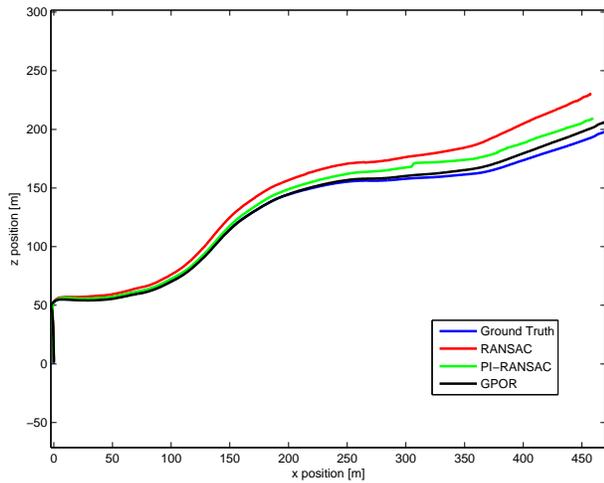
Fig. 4. Vehicle motion generated using visual odometry and outlier rejection techniques for S01.
