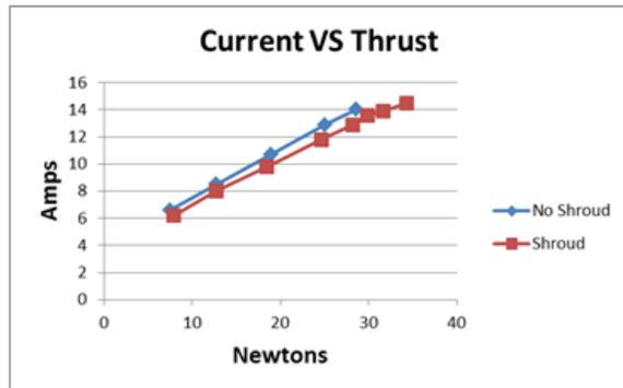
Figure 6 – Experimental data showing the electrical current drawn by the system for a given thrust, with and without the use of a duct. Current requirements are reduced when using the duct.
