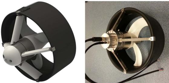
**Figure 14 – Solidworks rendering of the 3000W thruster along with a picture of its current state of assembly.**
