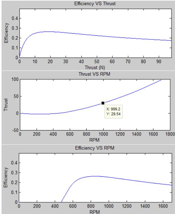
Figure 3 – These three graphs show simulated system performance data for a particular propeller geometry.
