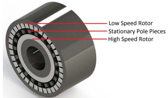
Figure 12 – A rendering of the magnetic gear topology used in the USC thruster. 4 magnets form the High Speed rotor and 34 magnets form the Low Speed rotor, resulting in a 1:8.5 gear reduction. 19 pole pieces provide flux harmony.
