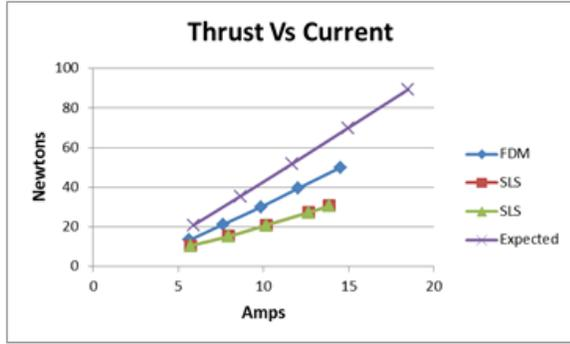
Figure 8 – Propulsion test results for propeller 2 along with its expected performance. Similar results were found for propeller 1.
