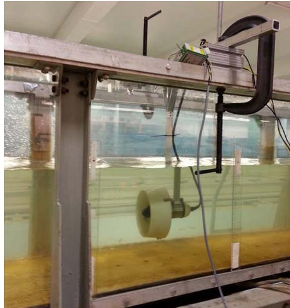
Figure 4 – Experimental setup of the 400W thruster within the open-water flume tank.
