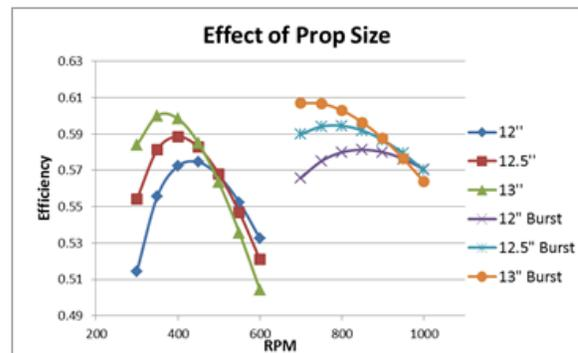
Figure 9 – Effect of propeller diameter on efficiency for cruise and burst operating modes.
