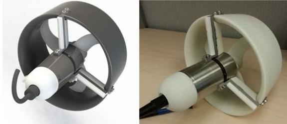
Figure 2 – A Solidworks [6] rendering of the 400W thruster and a photograph of the assembled unit.
