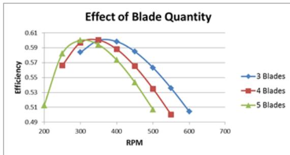
Figure 10 – The effect of blade quantity on propeller efficiency for a 13” propeller.
