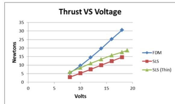
Figure 7 – The thrust generated by the three versions of propeller 1. Similar results were found for propeller 2.
