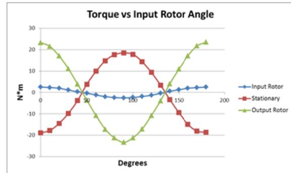
Figure 13 – COMSOL data showing the torque felt by each rotor. The output rotor can transmit 24 Nm before the gear will slip.
