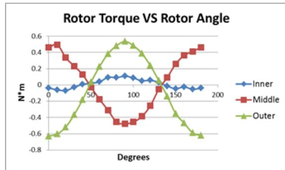
Figure 1 – COMSOL results showing the torque felt by each of the magnetic gear rings as the input rotor is rotated. Output torque peaks at 0.58 Nm.
