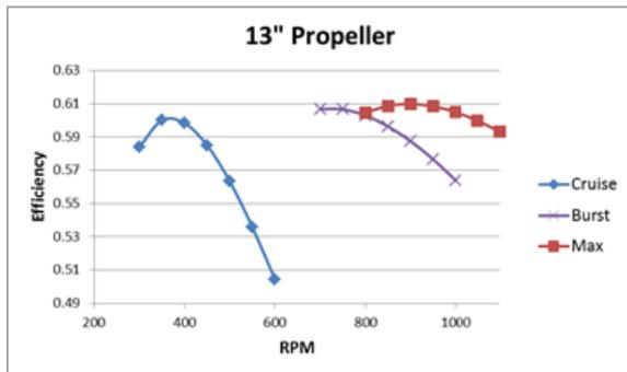
Figure 11 – Propeller efficiency versus rotational speed for each operating mode of a 3 bladed 13” propeller.
