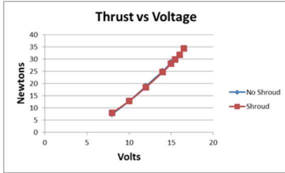
Figure 5 – Experimental data showing the thrust generated by the ducted and non-ducted propeller as the input voltage is increased. The thrust increase is considered negligible.
