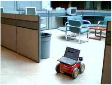
Fig. 2. A photograph showing the Pioneer robot used in experiments operating autonomously under laptop control. The forward facing monocular camera can be seen mounted on the front right-hand side of the robot.
