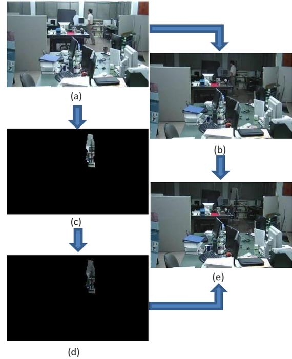
Fig. 5: Reconstructing the background model for an occluding moving object
