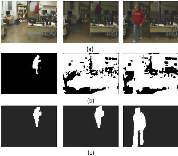
Fig. 6: (a) Samples of video frames, (b) Result from ALPCA and (c) Result of our approach
