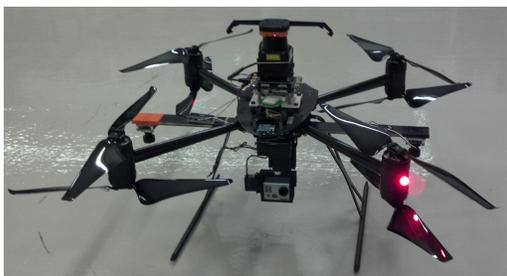
Figure 6: The *Draganflyer X8* retrofitted with LIDAR, beam directing mirrors and a GoPro camera.
