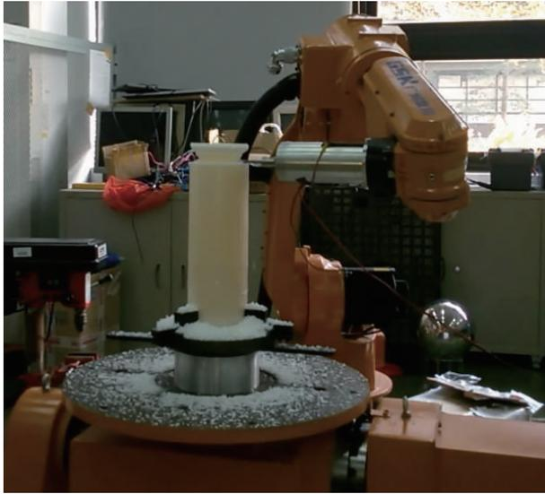
Fig. 10. Manipulator and positioner coordinating motion
